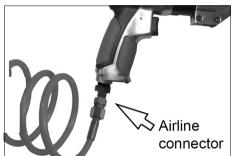
2. If a mini-oiler is not being used, run a few drops of oil through the tool before use. It can be entered through the inlet strainer or via the hose at the nearest connection to the air supply.
