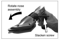
2. Ensure you have re-tightened the screw before using the shear.
